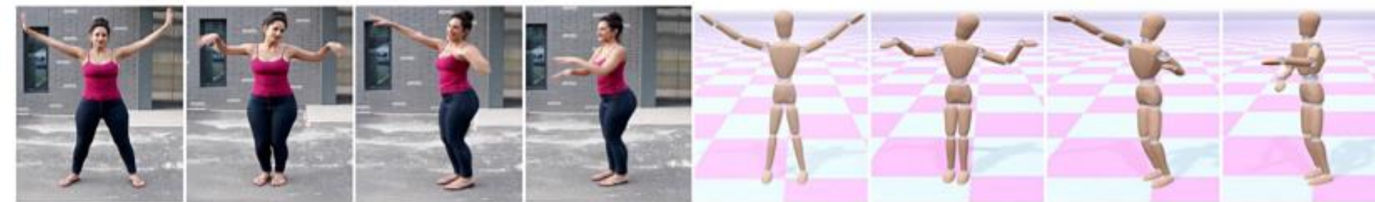
Fig. 1. Given a monocular video of a performer, our approach, MotioNet, reconstructs a complete representation of the motion, consisting of a single symmetric skeleton, and a sequence of global root positions and 3D joint rotations. Thus, inverse kinematics is effectively integrated within the network and is data-driven rather than based on a universal prior. The images on the right were rendered from the output of our system after a simple rigging process.
