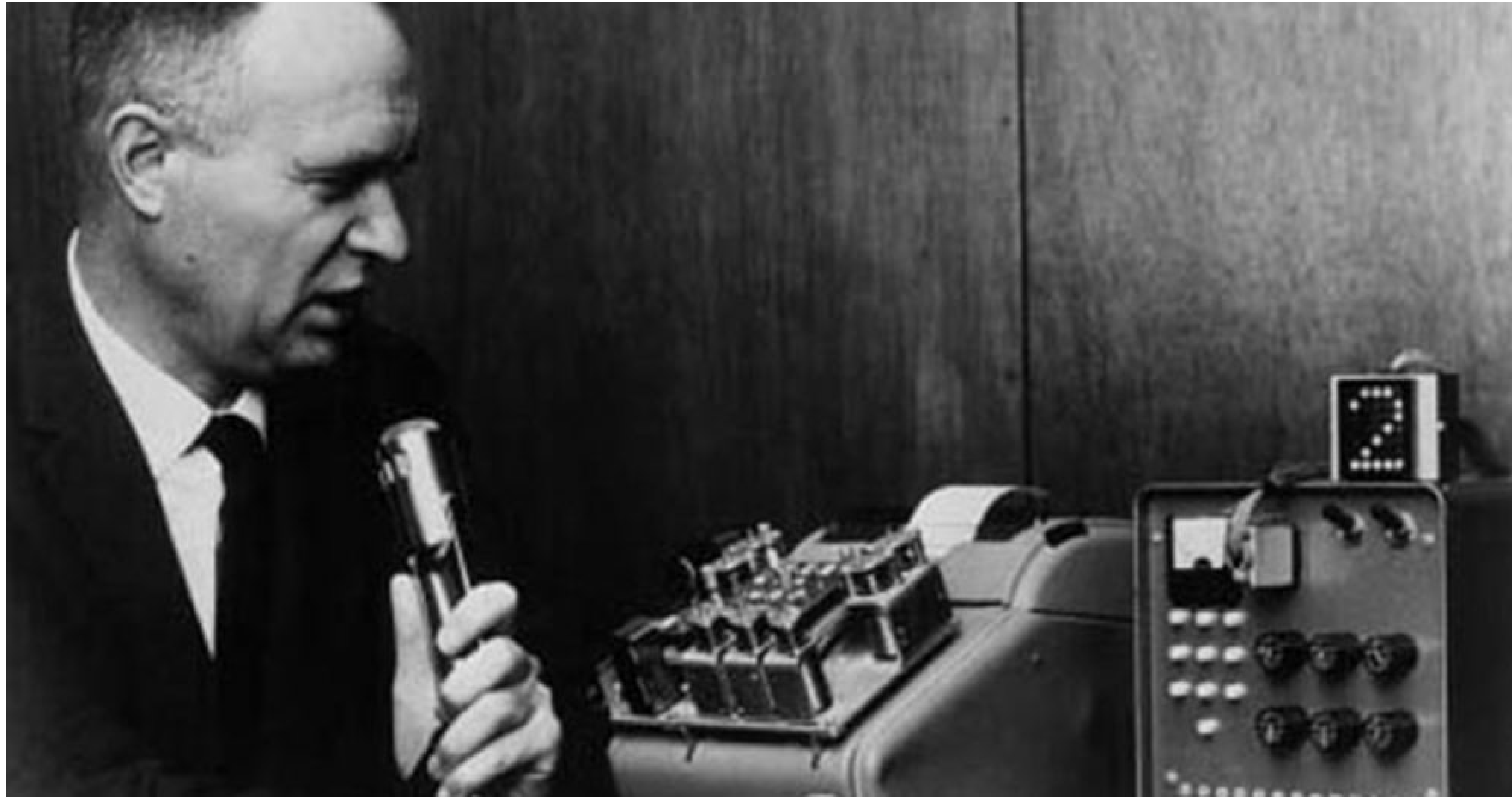
1952 Bell Labs Audrey. The photo shows only input and output controls but doesn't show supportive electronics. (Image credit: Computerhistory)
