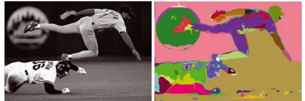
Figure 3. A baseball scene (432 × 294 grey image), and the segmentation results produced by our algorithm ( \sigma = 0.8, k = 300 ).
