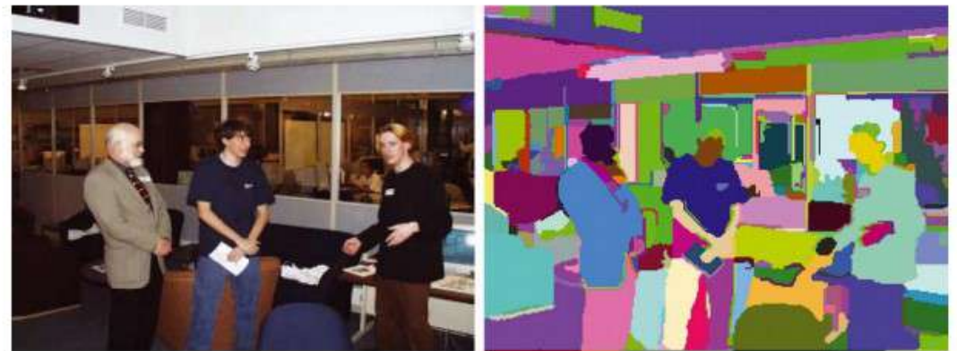
Figure 4. An indoor scene (image 320 × 240, color), and the segmentation results produced by our algorithm ( \sigma = 0.8, k = 300 ).
